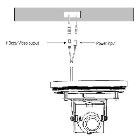
3. Fix the camera base to ceiling or wall by using 3 screws and washers. The washers are used to create the IP66 seal and must be used.
